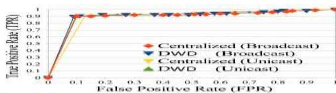
Fig. 11. The ROC diagram of Centralized Algorithm and DWD on networks with various topologies.
