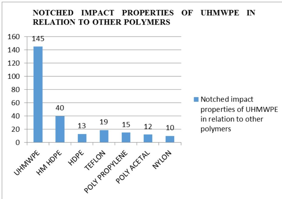
**Fig 3. Graph of Comparison of Notched Impact Strength of UHMWPE**
