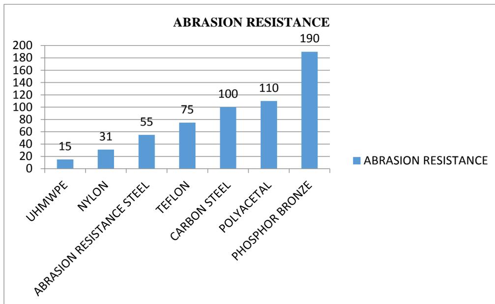
Fig 2. Graph of Comparison of Abrasion Resistance of UHMWPE
