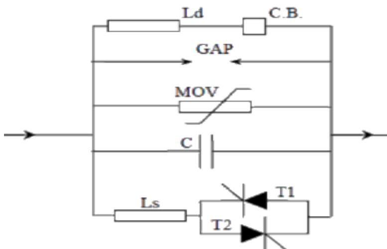
Fig.1 Basic Structure of TCSC
