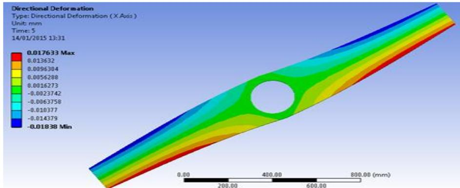
Fig.4 Directional Deformation on of flat agitator
