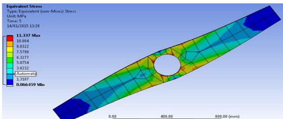
**Fig.3 Equivalent stress on flat agitator**
