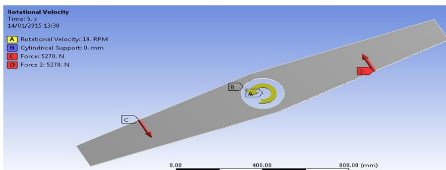
**Fig.2 Boundary conditions on flat agitator**
