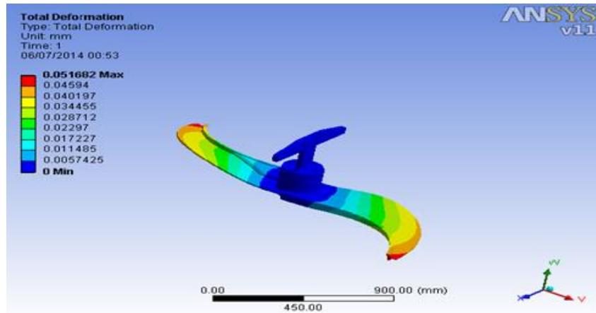
Fig.6 Total Deformation on S Agitator
