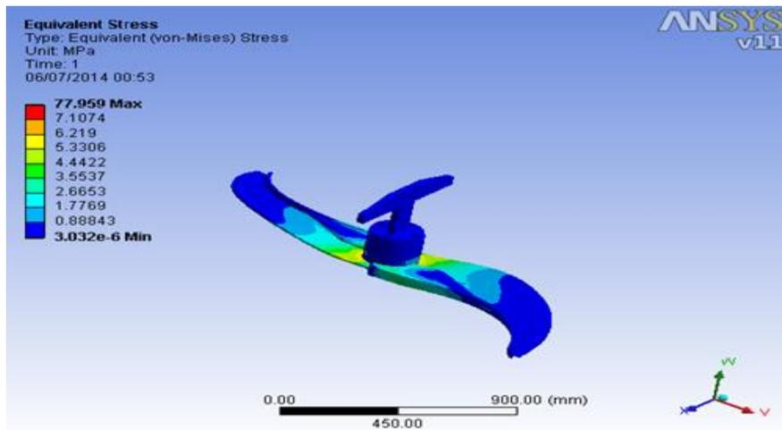
Fig.7 Equivalent stress on S Shape Agitator
