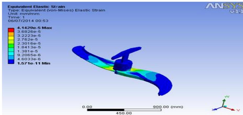
Fig.5 Equivalent elastic strain on S agitator
