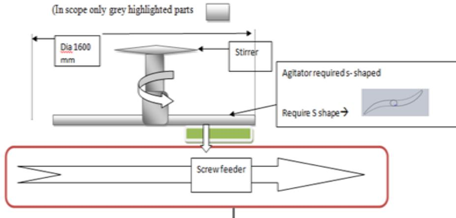
**Fig.1 Process layout of new agitator**
