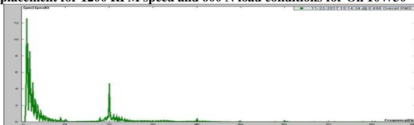
Fig.14 Graph of displacement for 1200 RPM speed and 600 N load condition for Oil 10W30
