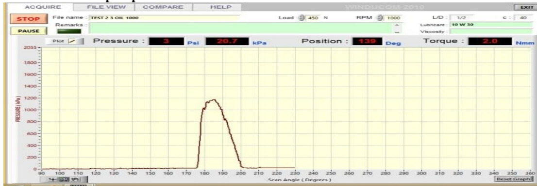
Fig.3 Variation of pressure with angular position and load condition at 1000 rpm and 450N Load Grade Oil SAE 10W30
