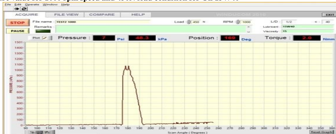
Fig.5 Variation of pressure with angular position and load condition at 1000 rpm and 450N Load Grade Oil SAE 15W40
