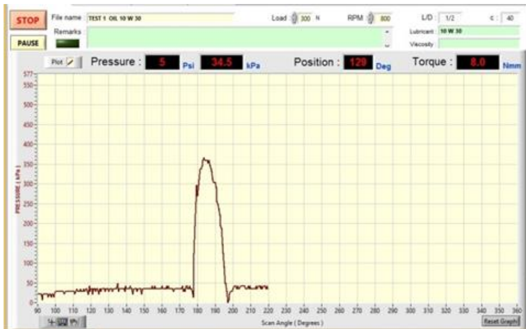
Fig.2 Variation of pressure with angular position and load condition at 800 rpm and 300N Load Grade Oil SAE 10W30
