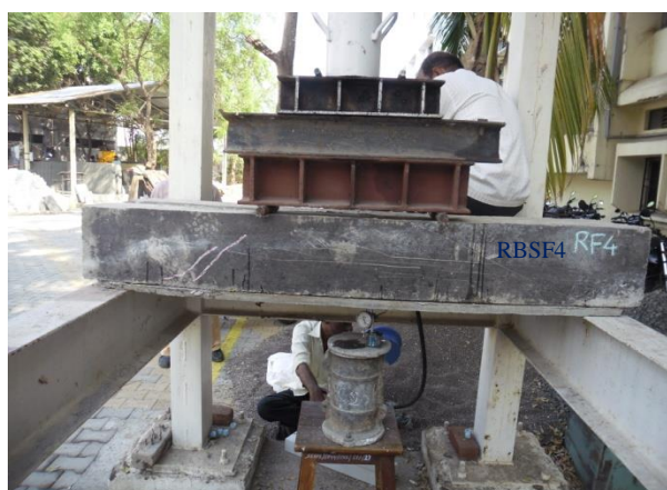
Fig.8 Compression cyclic loading setup of Control beams and SIFCON laminated beams.
