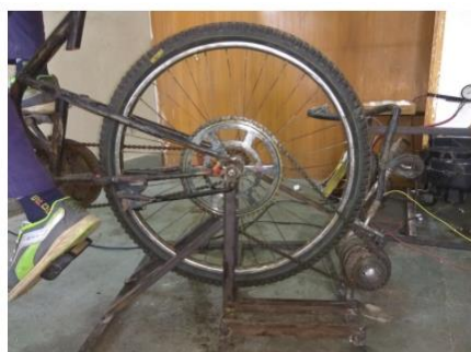
Fig.4 Chain Drive connecting with Compressor
