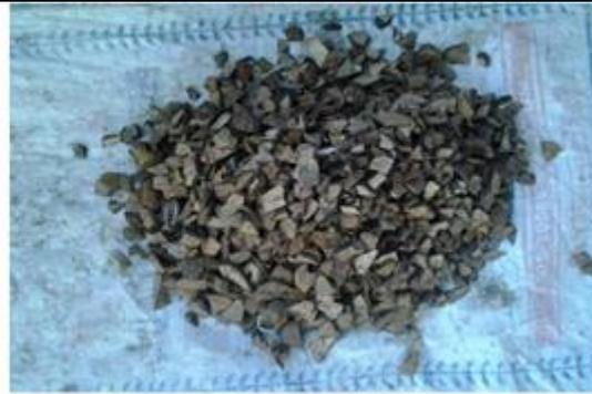
Fig.2 Coconut shell as aggregates
