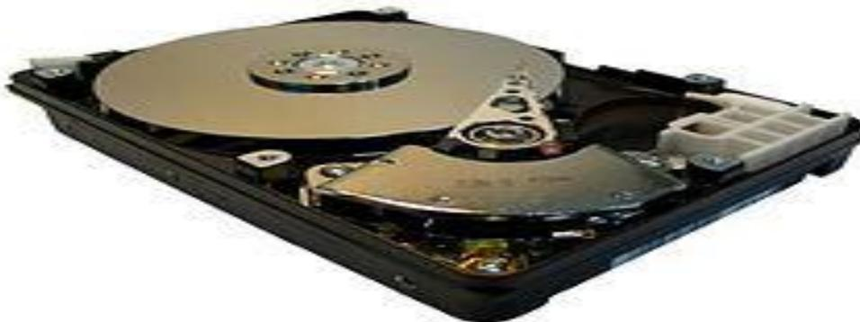
**Fig.4 Most hard disk drives incorporate strong magnets**
