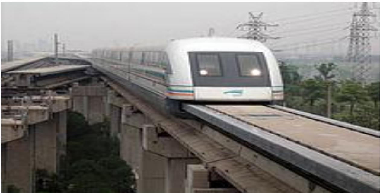
Fig.12 The Trans rapid system uses servomechanisms to pull the train up from underneath the track and maintains a constant gap while travelling at high speed
