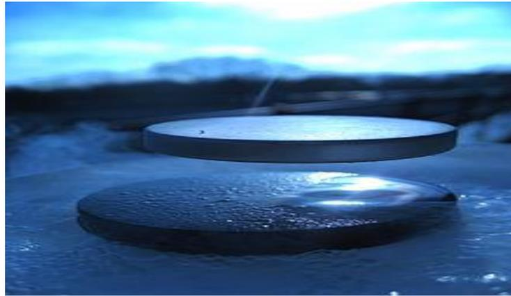
Fig.10 A superconductor levitating a permanent magnet
