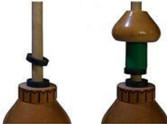
Fig. An example of magnetic levitation with a mechanical support (wooden rod) providing stability.
