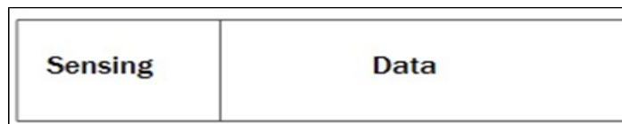
Fig. 3. Time slot structure, showing Sensing period
