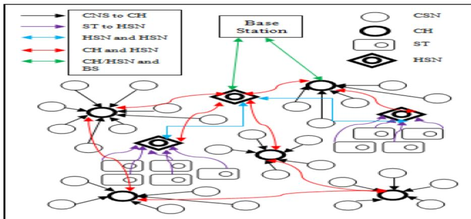
Fig.1. Architecture for Integration of WSN and RFID.
